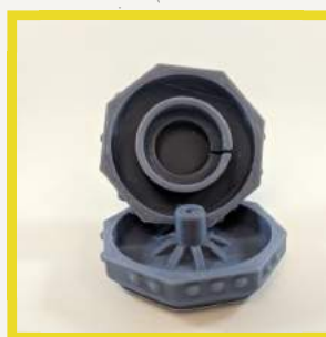
This print can help people learn to read braille! A bearing inserted around the center pin allows the outer shells to rotate, representing each letter of the braille alphabet
